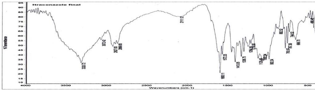
Fig 4: FTIR spectra of Itraconazole optimized formulation
